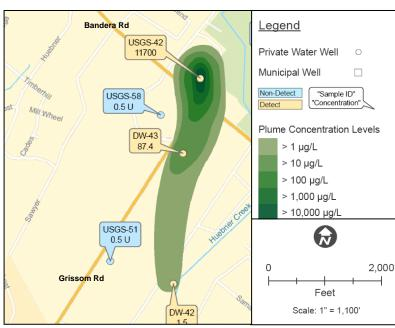
Figure 4. Tetrachloroethene (PCE) Ground Water Sampling Results (July 2008). From EPA's updated Conceptual Site Model (Attachment I - Figure I-4). Maximum concentrations from samples are shown. These samples were collected in January 2008 through passive diffusion bags in private water wells. Sample results and chemical concentration amounts are presented in micrograms per liter ( $\mu$ g/L). EPA's MCL for PCE is 5  $\mu$ g/L.
