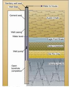
Figure 1. Diagram illustrating the components of a ground water well. Source: Edwards Aquifer Authority. The typical well construction near the Bandera Road site is "open hole" (uncased) in the water bearing zone. The well pump may be set either within the uncased section of the borehole or within the well casing.
